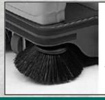
The side brushes are activated via ergonomic controls accessible from the operator's position. The shock resistant supports avoid damage which could be caused by accidental impact. The second, left side brush, is available as an optional.
