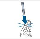
1. Insert handle into body of machine until it clicks into place.
